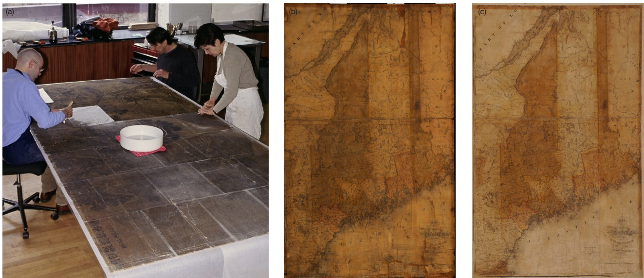
Fig. 4 (a) Use of usukuchi rayon paper (18 gm 2 ) facings for cleaning and reinforcement, with additional support provided by thick rayon paper (50 gm 2 ) and Melinex, during backing removal, filling and lining. Wall map Maine (1872), intaglio printed and hand coloured. (b) Before and (c) after treatment.
