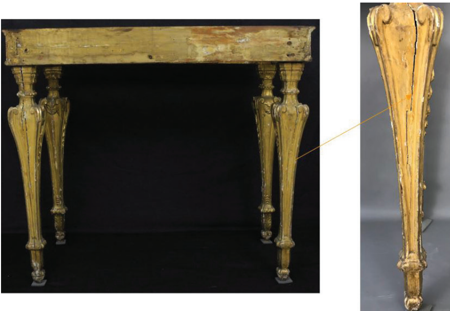
Fig. 25. An example of splits in the legs at the back of the table.
