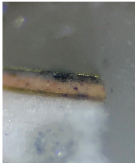
Fig. 27a. Sample from the front leg, 200x magnification. 1-gesso, 2-red bole, 3-gold leaf, 4-pale red bole, 5-gold leaf, 6-grey bole, 7-gold leaf.
