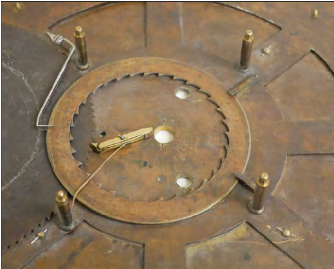
Back of the dial showing the large gaps in the dial plate – a feature of Northern English clocks
