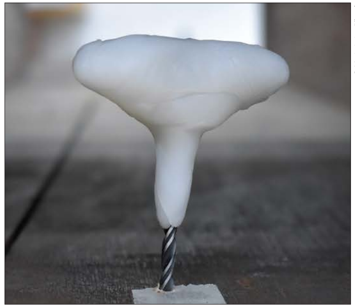
To drill the holes for the screws fixing the batten to the spine the creation of a bespoke drill handle made from Polymorph (a thermoplastic polymer) was necessary due to the limited space inside the carcass
