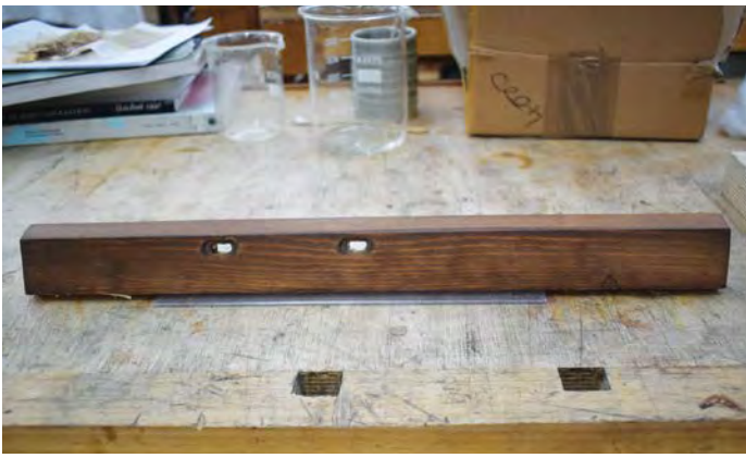
The batten introduced to the bottom of the spine (the boards forming the back of the clock case) to increase the stability of the construction
