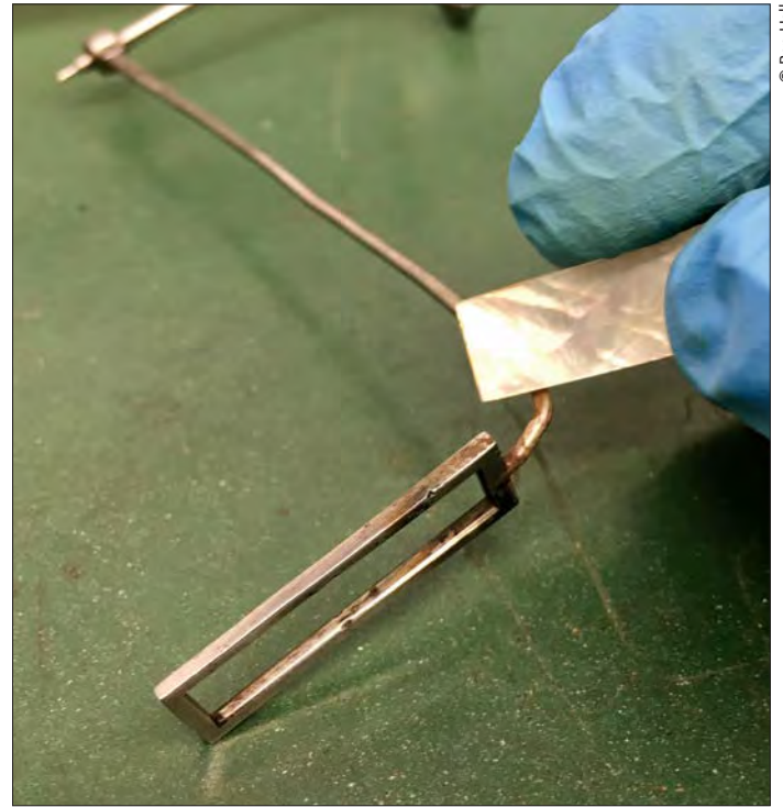
After the clock's movement was disassembled, a mother of pearl scraper, amongst other tools, was used to remove corrosion and rust from steel parts
