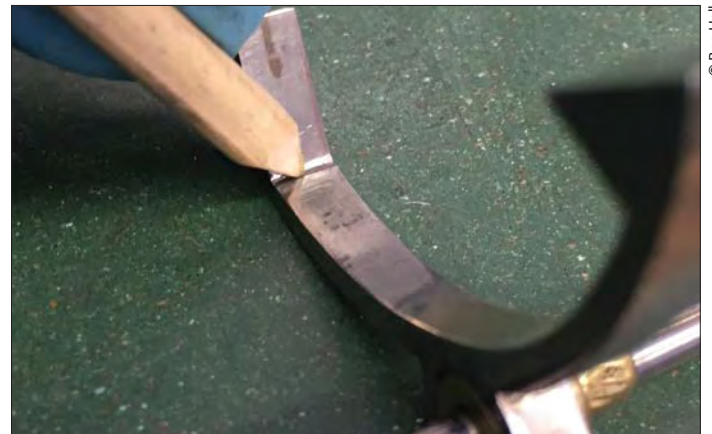
Manual cleaning of the movement's components using peg wood to remove hard oil deposits and dirt
