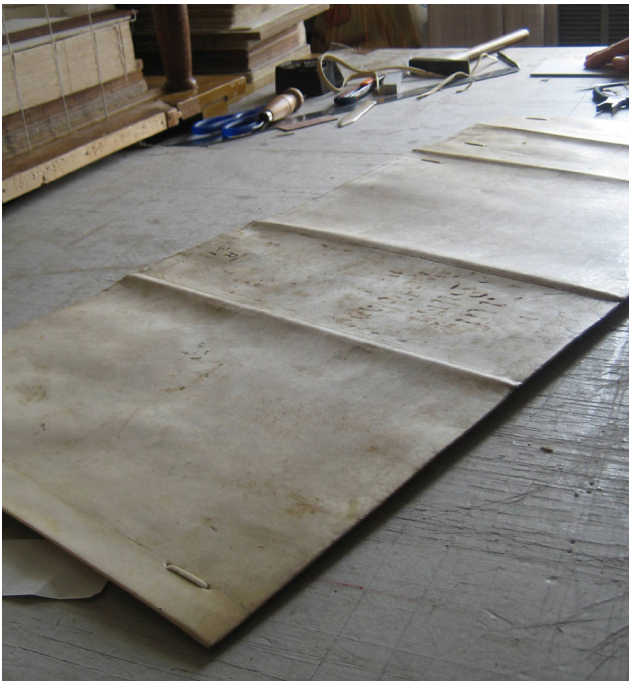
Fig. 3 The external structure of the new vellum binding showing the folds tackets at turn-ins. Grottaferrata conservation studio & bindery.
