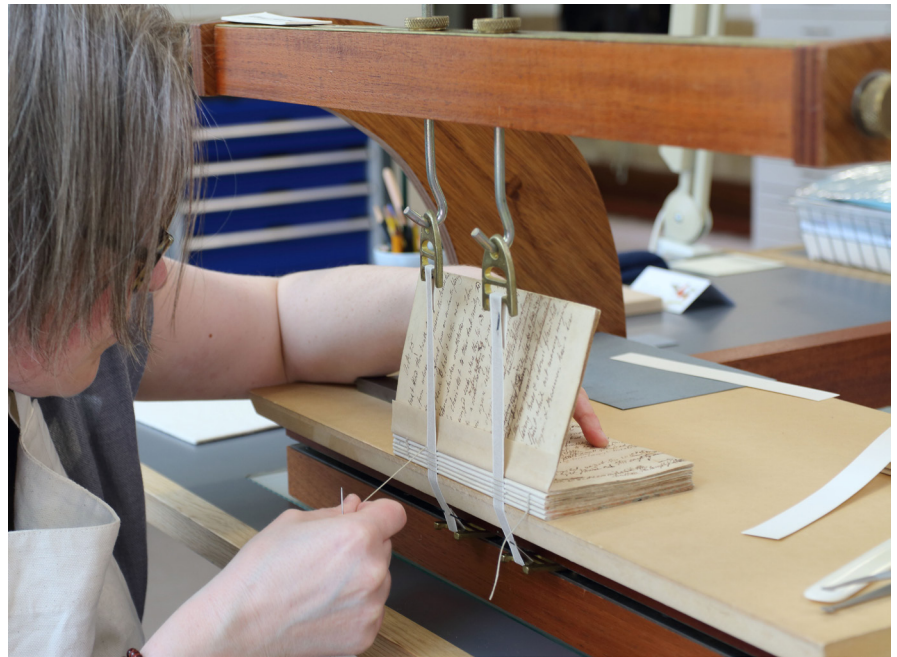
Fig. 6 Sewing the bookblock on two linen tape supports. (Bodleian Libraries, University of Oxford, MS. Shelley adds. e. 12)
