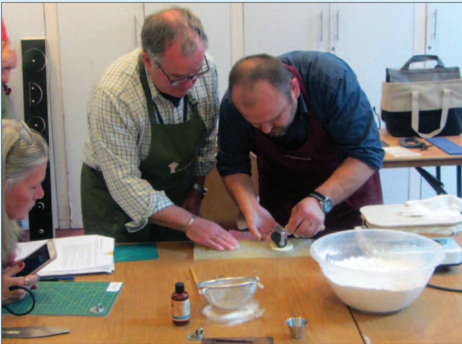
Pressing compo, using traditional boxwood moulds
