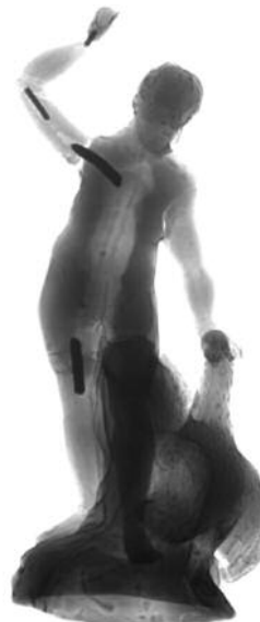
Image obtained using X-ray radiography operated at 70 kV, 2 mA current with a 0.01 second exposure
