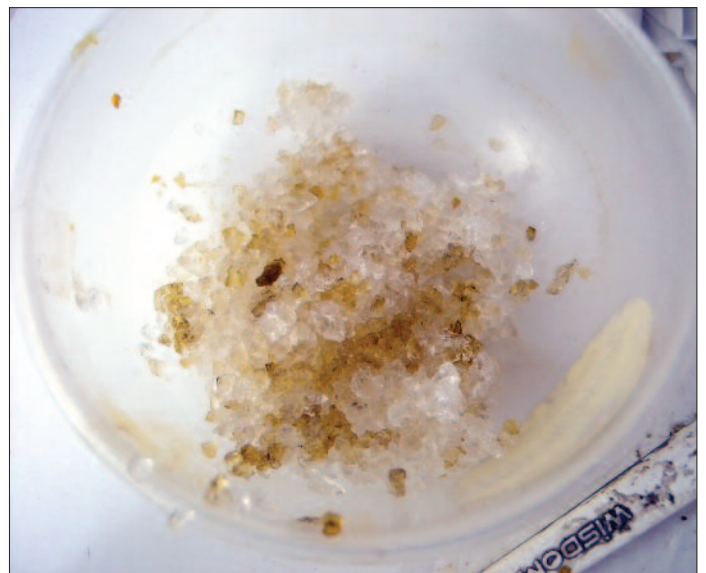
The discoloured SwellGel after its removal
