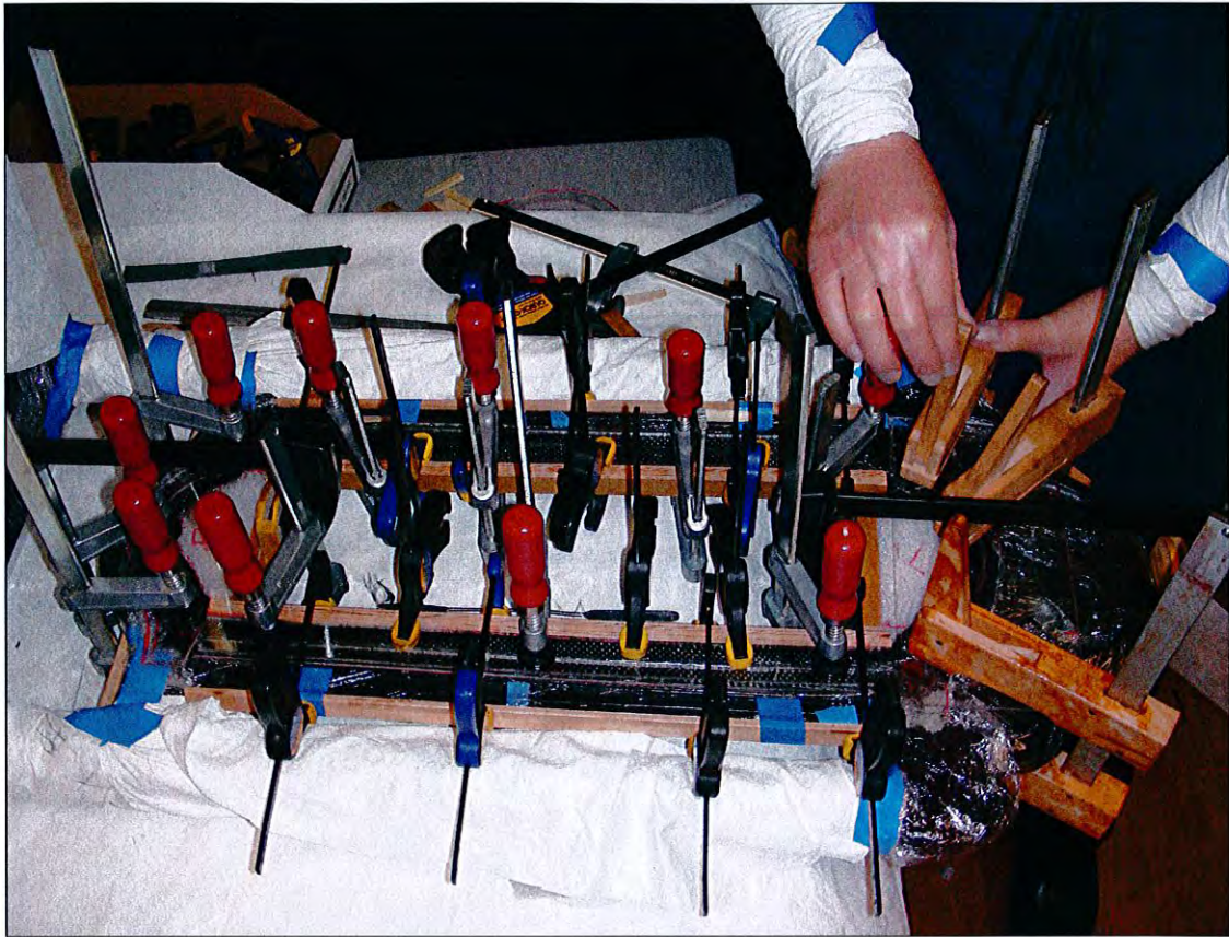
Fig. 5: Back carbon fiber cast with clamps in place
