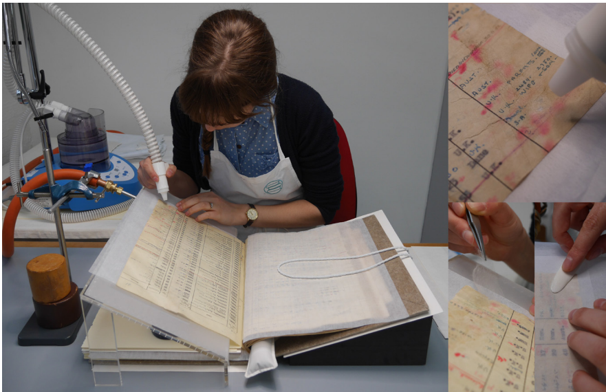
Fig. 7 (clockwise from left) Applying isinglass adhesive and tissue to a leaf of the nominal roll on the Perspex frame with the suction wedge held behind with a laboratory stand, detail of adhesive vapour, detail of silicon paper and bone folder, detail of Berlin Tissue. Courtesy of Emma Nichols, Conservation Department, Cambridge University Library. RCMS 103/12/22.
