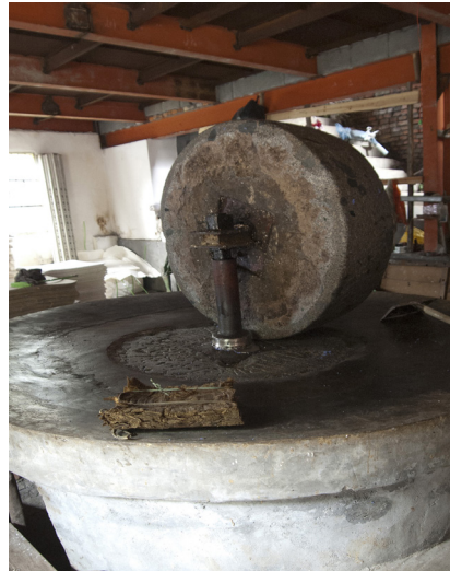
Fig. 1 Grindstone used for preparing fibre pulp, Yuanshu (Zhejiang province), China. Image copyright C. Laroque.
