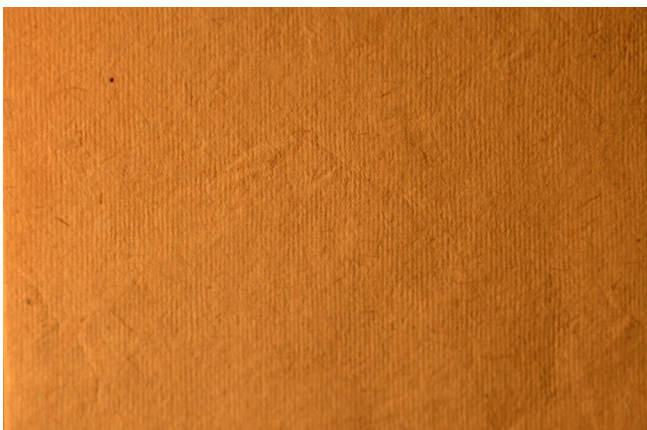
Fig. 4 Imprint of Indian woven paper formed on a mould with textile sieve. Image copyright C. Laroque.
