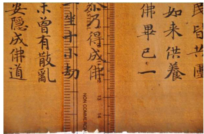
Fig. 5 Imprint of Chinese laid regular paper formed on a mould with movable net. Image copyright A. Helman-Wazny.
