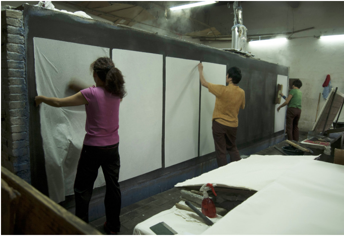
Fig. 2 Paper drying on heated walls, Fuyang (Zhejiang province), China. Image copyright C. Laroque.
