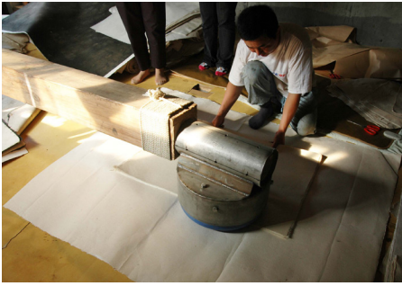
Fig. 14 Hammering of paper or dochim , Gyung Gi, Korea. Image copyright C. Laroque.
