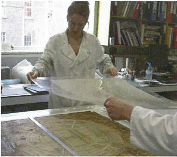
Figure 7 Casting prepared paper to reverse. © The Trustees of the Chester Beatty Library, Dublin
