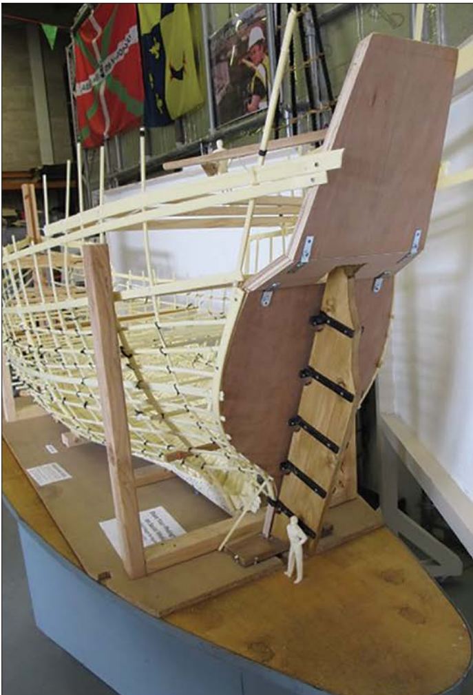
Each timber was recorded using contact digitisers and this highly accurate geometric data was converted into digital solid models which were 3D printed and assembled to form a 1:10 scale model of the recovered hull.
