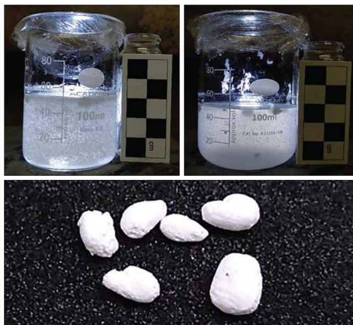
Fig 2 .Results of solubility tests after 1 hour - Dimethyl Carbonate (top left), Ethyl Acetate (top right) and white balls sampled from Ethyl Acetate (above)
