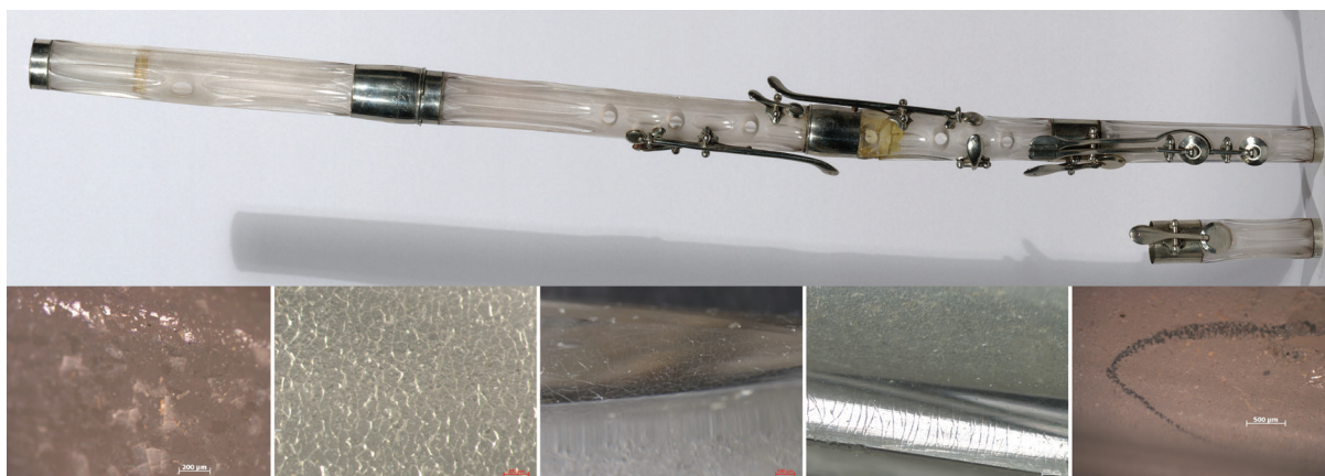
Figure 1. Claude Laurent, Flute in C, ca. 1815 CE, glass, silver, mother-of-pearl, L 61.7 cm × W 66.9 cm. Library of Congress, DCM 717 · Courtesy of Library of Congress · Photomicrographs of DCM 717 (below, left to right): exterior of head joint, cracking and spalling; interior of head joint, severe network cracking; exterior of foot joint, fine network microcracking; interior of extra foot joint, fine, parallel microcracking; interior of extra foot joint, rough polished surface with no visible deterioration
