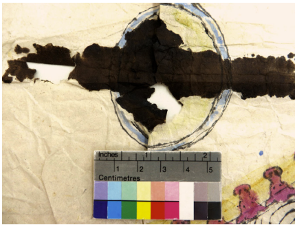
Fig. 5 Detail of one damaged area, in which a major fold is stuck. The damaged paper is only sticking together locally. München, Bayerische Staatsbibliothek, Cod.tibet. 992.
