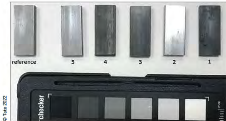
Steel strips at stage 1 (start date on 15 April) corrosion test after 1 month. 1 - instant coffee; 2 - Van Dyke Brown crystals in DI; 3 - Dark soy sauce; 4 - Balsamic vinegar; 5 - Engine Oil (for testing solvent cleaning only)
