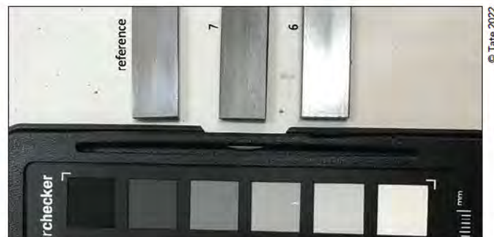
Steel strips at stage 2. Corrosion test after 1 month. 6 = Glycerin + Van Dyke Brown in DI; 7= Glycerin + Van Dyke Brown in DI + dark soy sauce
