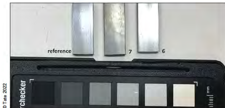
Steel strips at stage 2 (start date on 7 Jun) corrosion test after 2 weeks. 6 = Glycerin + Van Dyke Brown in DI; 7= Glycerin + Van Dyke Brown in DI + dark soy sauce
