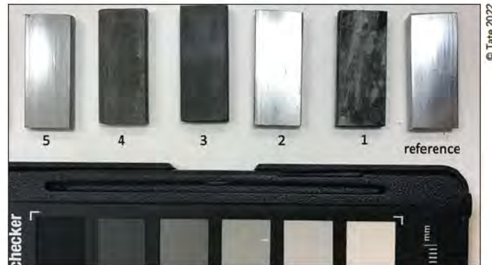
Steel strips at stage 1. Corrosion test after 2 months. 1 - instant coffee; 2 - Van Dyke Brown crystals in DI; 3 - Dark soy sauce; 4 - Balsamic vinegar; 5 - Engine Oil (for testing solvent cleaning only)
