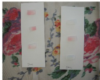
Image 6. The six gel blocks after testing with visible signs that the gel had taken up dye.
