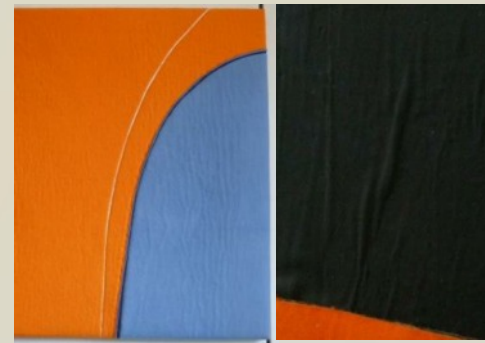
Fig. 3. Serious delamination issue of all the layers of a panel, obverse and reverse of a panel.
