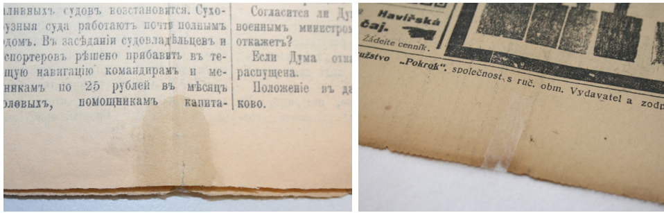
Fig. 17, a The use of wheat starch paste and remoistenable tissue on Russian newspapers, 1916–18, Collection of the International Institute of Social History, Amsterdam. Photo: RNA.
