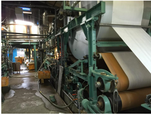
Fig. 2 Kentsuishiki papermaking machine at the calendaring and drying section, Hidakawashi paper mill.
