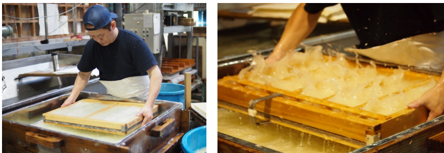
Fig. 1 Handmade tamezuki process, Awagami factory. To overcome the bias of causing fibres to orientate themselves parallel to the short side of the mould, the vatman shakes the screen between two perpendicular directions. This produces a sheet with no apparent directionality, in contrast to the nagashizuki method.
