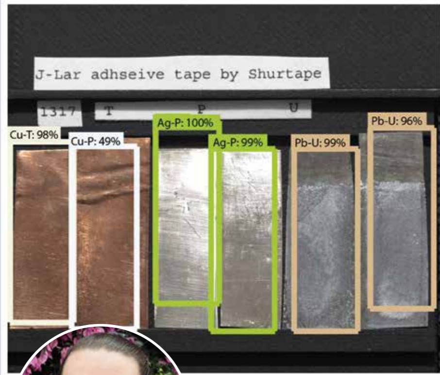
Above: The trained CNN correctly identified the metal and corrosion level of 98% of the coupons in a test set of images
