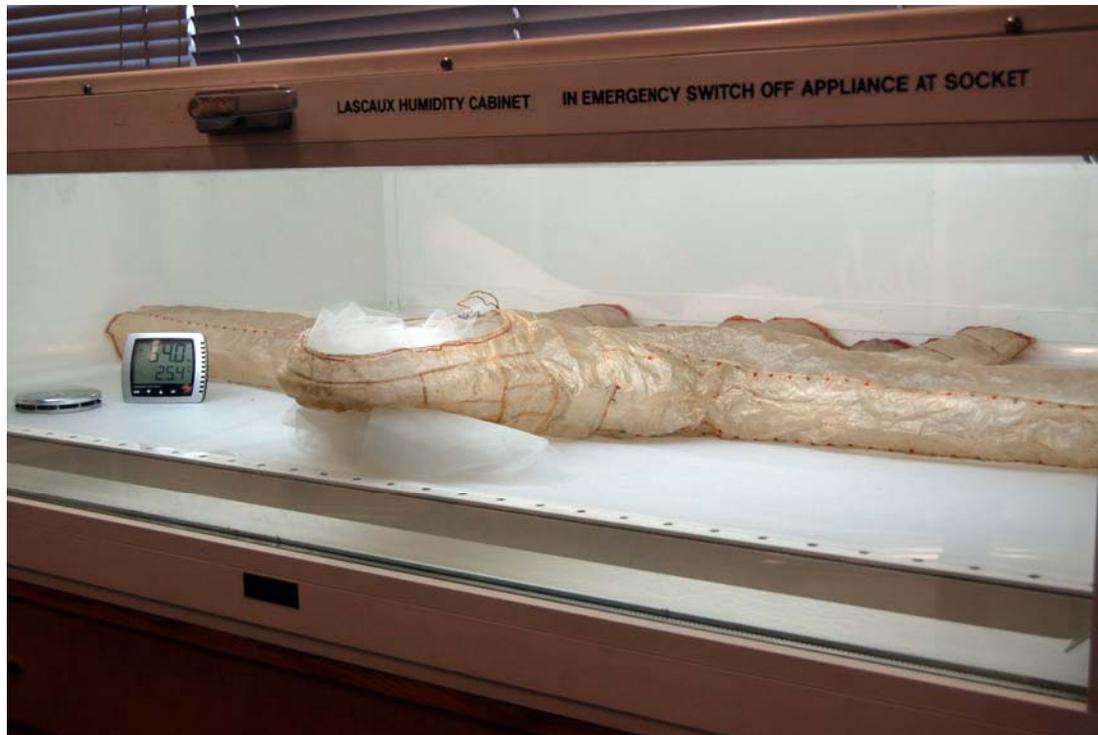
Figure 2. Padding out with crumpled nylon net during humidification in humidity cabinet. ©The Trustees of the British Museum.
