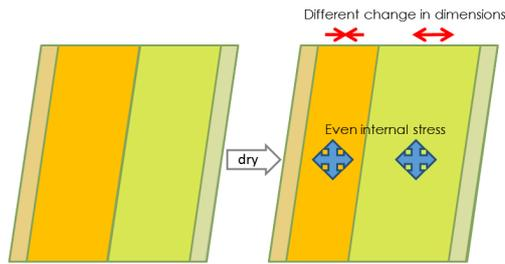
Fig. 2 Dimensional change (red arrows) and internal stress (blue cross arrows) during karibari.
